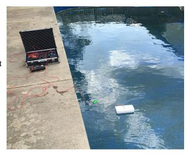
2) Using the LT1000 Amp and PoolScope, listen to all penetrations, step channels, lights, skimmers, main drains, side suction around lights, spas, etc. This procedure will find leaks or rule out these areas. This step cannot be done with the VILO.
