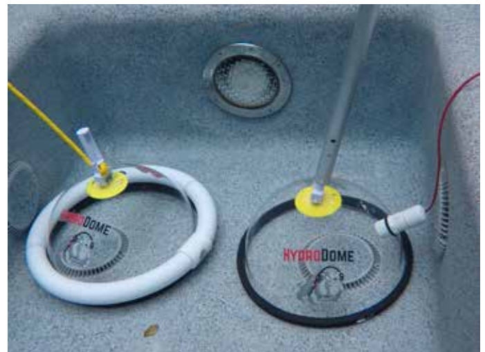
The listening and seal domes over a spa dual drain system.
